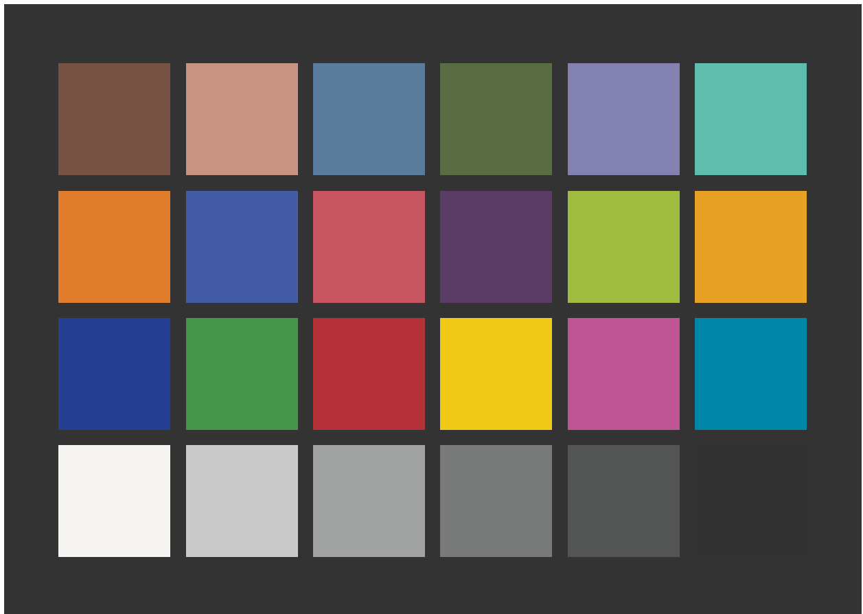
Figure 6: Rendering with Illuminant D65 and xyz1931.1nm, at age=64 after chromatic adaptation
