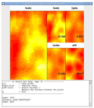
This function also has an argument named panel.last, which allows to pass an expression to be evaluated after plotting has taken place. For example, we can use it to explore the distribution of lynx indices in relationship with the maps. Copy and paste the following expression:
